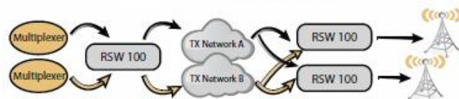
Dual transmission on paths from multiplexer site.
